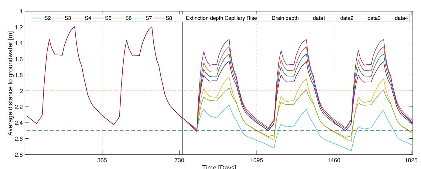
Conjunctive use of surface- and groundwater through the operation of drainage pumps and canal leakage reduction of 50% is the most effective mitigation scenario.
