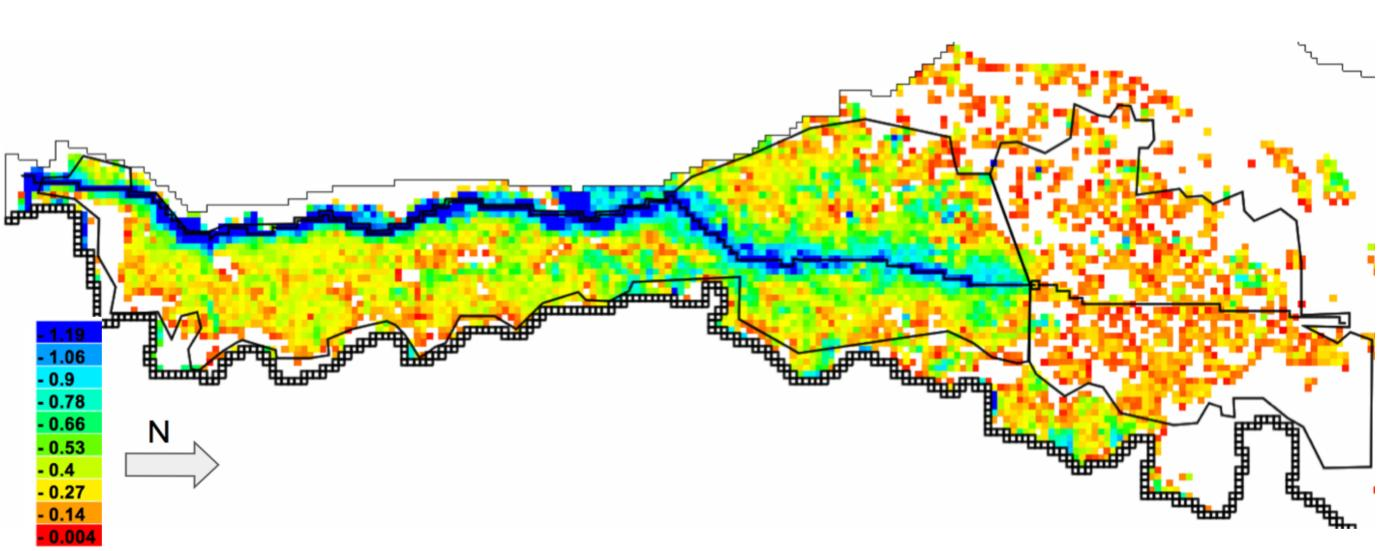
Spatial distribution of capillary rise rates in mm/day. Green blue colours indicate high rates that are mainly driven by very shallow groundwater tables and insufficient drainage.
