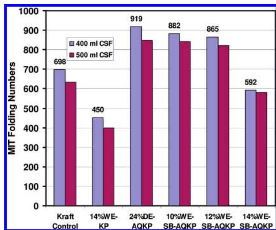
Figure 15. MIT folding endurance of 14%WE-KP, 24%DE-AQKP, and 10, 12 and 14%WE-SB-AQKP and control compared at 400 and 500 mL CSF.
