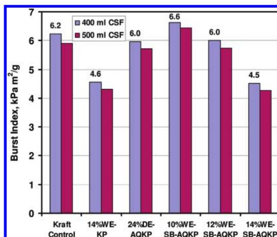
Figure 13. Burst index of 14%WE-KP, 24%DE-AQKP, and 10, 12, and 14%WE-SB-AQKP and control compared at 400 and 500 mL CSF.
