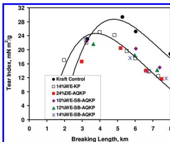
Figure 14. Tear index versus breaking length of 14%WE-KP, 24%DE-AQKP, and 10, 12, and 14%WE-SB-AQKP.
