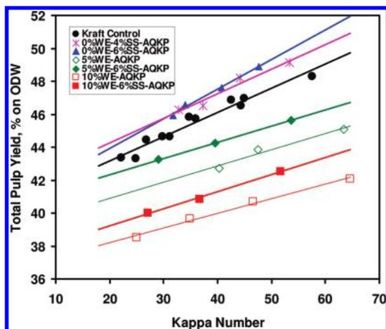
**Figure 4.** Total pulp yield vs kappa number for kraft pulping of water pre-extracted wood chips (5% and 10% weight loss) compared to that of regular kraft cook.
