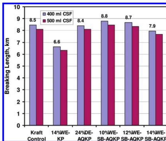
Figure 12. Breaking length of 14%WE-KP, 24%DE-AQKP, and 10, 12, and 14%WE-SB-AQKP and control compared at 400 and 500 mL CSF.
