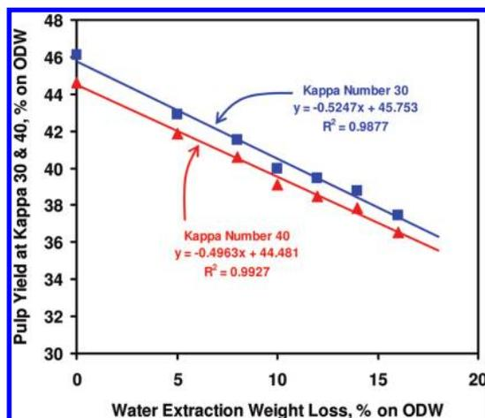
Figure 3. Total pulp yield versus weight loss for kraft pulping of water pre-extracted wood chips compared to kraft control at kappa number 30 and 40.
