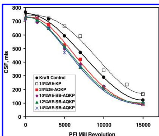
Figure 11. Plot of pulp freeness (CSF) versus PFI mill revolution for modified kraft cooks with 10, 12, and 14% water-extracted wood chips and control.
