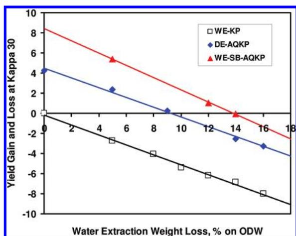
Figure 7. Yield gain and loss diagram for water extraction followed by kraft pulping (WE-KP), double extraction and AQ-kraft pulping (DE-AQKP), and water extraction followed by sulfide-borohydride treated AQ-kraft pulping (WE-SB-AQKP).
