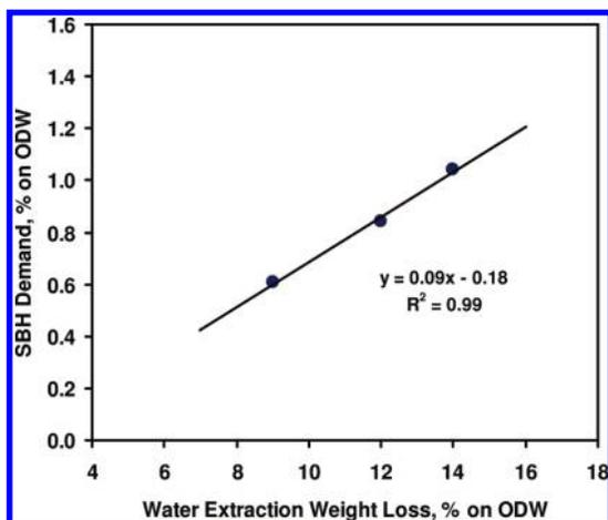
Figure 10. Plot of SBH demand for zero-yield-loss for kraft pulping of water-extracted wood chips versus water-extraction weight loss.
