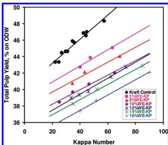
Figure 2. Total pulp yield versus kappa number for kraft pulping of water pre-extracted wood chips (WX) compared to kraft control.
