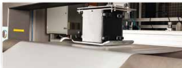
Automated Backsheet thickness measuring - RenewSys Bengaluru
