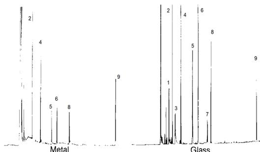
Figure 1. Polar Test Solution on Glass and Metal Systems
