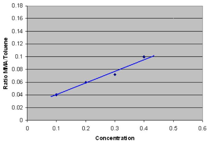
Figure 3. MMA/Toluene peak area ratios vs. MMA concentration.
