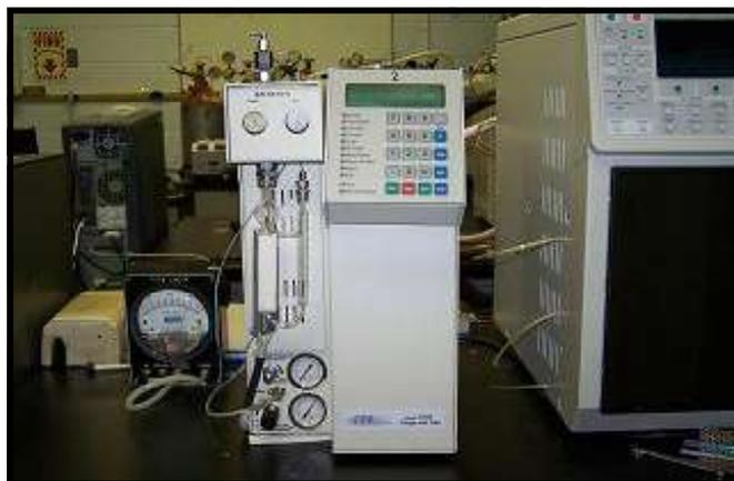
**Figure 3.** CDS 7000 with optional heater.
