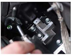
**3**. Fuel pressure valve can now be seen after removing Glow Plug Controller assembly. Unscrew valve and remove from fuel rail. Photo shows valve loosen and unthreaded most of the way.
