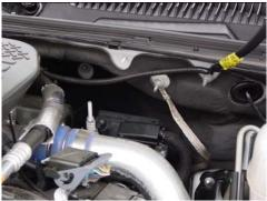
**2**. Remove the 5 bolts shown, four on the case and 1 on the metal tubing shown.
