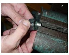
**7**. Removing the metal spring, then insert the 3 supplied metal shims into valve. Now re-insert the metal spring back into the valve.
