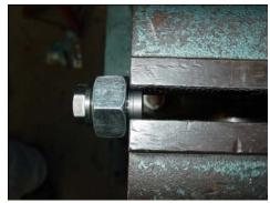
**5**. Use a wrench to unscrew supplied nut in order to remove valve cap. Be careful to hold end of valve while doing this! It is spring loaded and you don't want to loose parts! There is a small needle valve in the cap, it is located behind the washer with the 3 holes. Be sure it does not fall out. If it does the truck will not start once the valve is re-installed. If it does fall out be sure to re-install it. It is tappered and should be flush with the cap when inserted properly.
