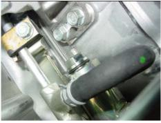
**4**. Take valve and thread supplied nut tool onto valve.
