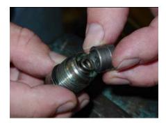
**9.** Place valve back in vice, now with a thick piece of cardboard or piece of wood behind valve cap to prevent damage to the valve seal surface. Tighten vice so that the valve cap reenters valve until fully seated. No need to over-tighten; just tighten until snug.
