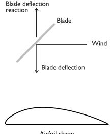
Airfoil shape (blade cross section)
