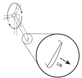
airfoil shapes over the years in an effort to find the perfect shape that will perform well in a range of wind speeds. Even minor changes in this blade shape can dramatically affect the power output and noise produced by a wind turbine. To get some ideas about different airfoils used in airplane wings and wind turbine blades, research the United States National Advisory Committee for Aeronautics (NACA). This group was responsible for designing a wide range of airfoils in the 1940s.
