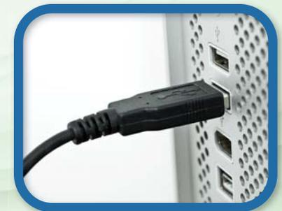
Start by inserting the USB cable into an unused USB port on your computer. No separate power connections are necessary.
