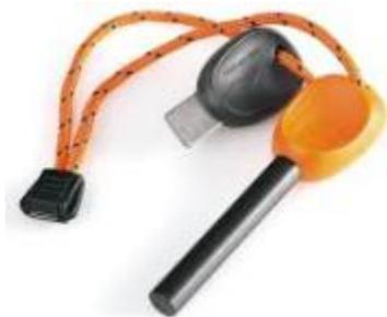
Traditionally a flint and steel were used; however, the flint was not the important part. With a proper striker, you can get sparks using any hard, non-porous rock that has a sharp edge, even petrified wood. The spark comes from chipping small pieces of steel off the striker; finely divided metals ignite immediately in air, with steel burning at yellow-white heat.
