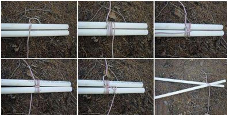
A shear lashing is often used to bind adjacent poles together. It is also a good way to reinforce a broken or weak pole. The frapping turns used to tighten the lashing may be omitted and replaced with wedges inserted between the poles.
