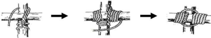
The square lashing to fasten two spars or poles together.
