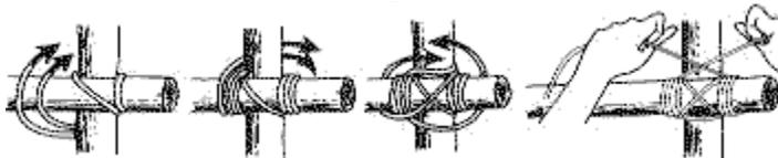
A lashing used in lightweight construction work. It is equivalent to a square lashing and when done correctly should be just as strong. End the lashing with a square knot.
