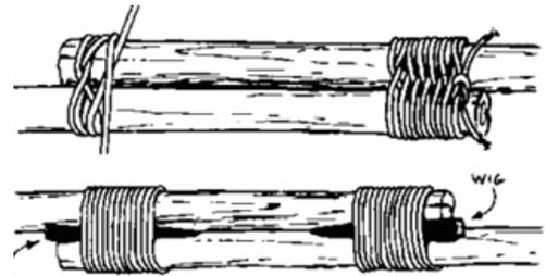
Used to lash two poles together (constructing a flagpole). Tie a clove hitch around the bottom pole. Wind the rope around both six or seven times. Finish with two half hitches around both poles. The lashing can be tightened by driving a small wooden peg between the poles. If possible force a wedge under the lashings to make them tight. If the spars are vertical, bang the wedge in downwards.
