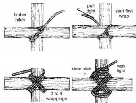
Tie a timber hitch diagonally around both poles.
