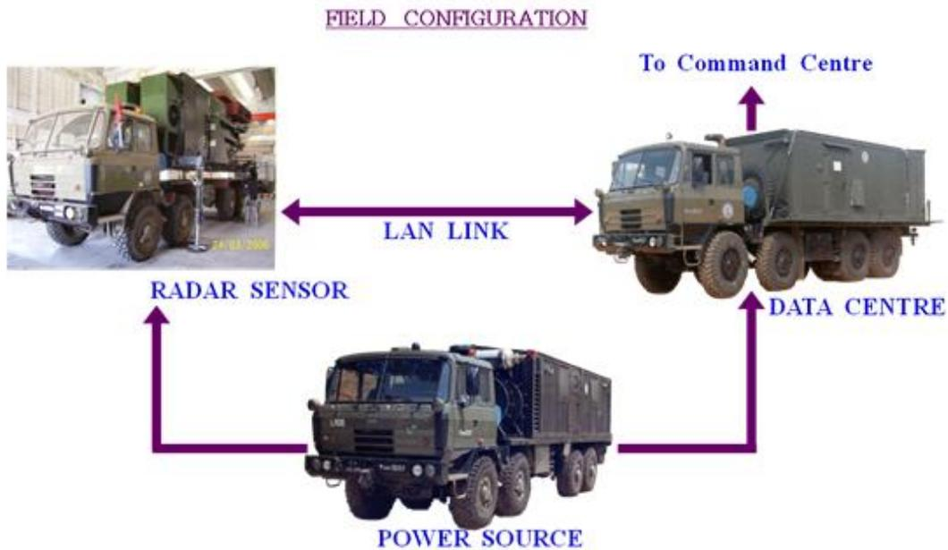
**Fig 2.1 Field Configuration for ROHINI Radar System**
