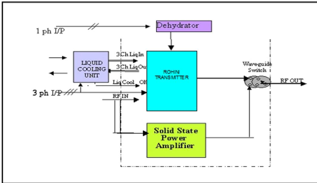
Fig. 4.1 Block Diagram of a Transmitter
