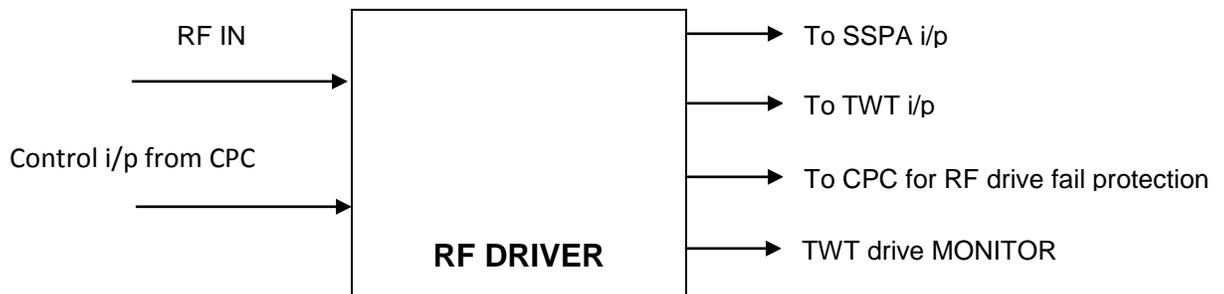
**Fig. 4.2 Input/output diagram of RF Driver**
