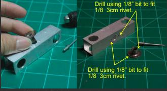
Using a 1/8 bit, drill 2 holes on the bottom of the tube. Align these with the 2 holes on the tee nut. Do this by fitting the tee nut into the 5/16" hole first, clamping it down then drilling through the holes of the tee nut as a guide.
