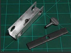
Don't forget to file down the edges of the finished rail block prevent cuts and injury.
