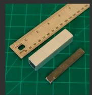
Also with the flat bar, cut an 8cm piece with the hack saw.
