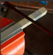
Using a hack saw cut an 8cm piece of the aluminum tube.
