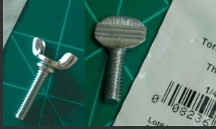
Choose between a winged screw left, or a thumb screw on right as a fastener to hold down the flat bar. I use both at 1/4 diameter and 3/4 length.
