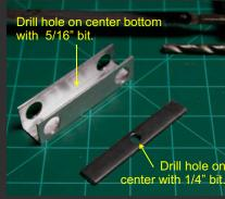
Cut off the top of the tube and drill a hole on the bottom center for a 1/4" tee nut to go through. Drill also the center of flat bar.
