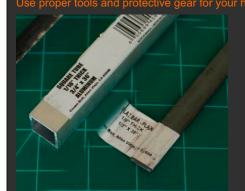
Square aluminum tube 1/16" thick 3/4" sides and steel flat bar 1/8" thick 1/2" wide.
