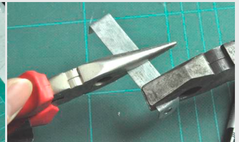
Cut a thin metal strip, this will be the lock that shall hold the pieces together.
