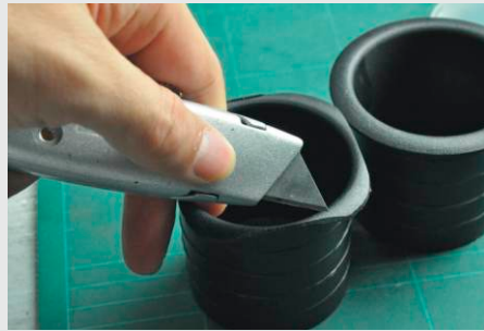
Trim the rim on one of the black cylinder (B) so it will slide into the top opening of the plastic container (A).
