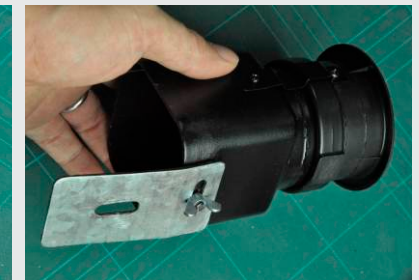
The mount plate is held in place by a winged nut for easy adjustment. The rubber padding helps the finder stay in place. The other side is not padded since most quick release plate is padded.
