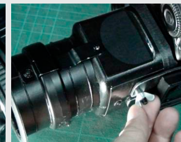
To quickly remove the loupe to view LCD, just loosen the wingnut.
