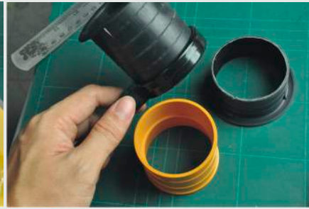
This vent (B) fits snugly inside the loupe rim, the PVC coupling might need a little trimming around the rim as this has a thick rib. The loupe handle is cut off at the base.
