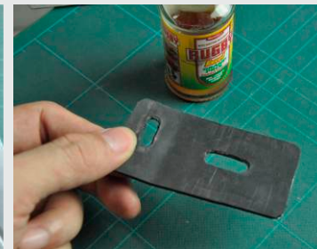
For our mounting plate, cut a thin metal sheet 80 x 45mm. Cut 2 elongated holes for adjustment when mounting. On one side of the mount plate, glue a thin rubber sheet. I cut out mine from an old motorbike innertube.
