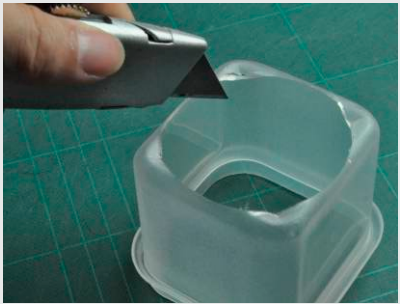
Cut a hole on base of the container (A) so the black cylinder will slide thru snugly.
