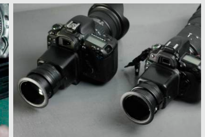
The mount plate is held in place by a winged nut for easy adjustment. The rubber padding helps the finder stay in place. The other side is not padded since most quick release plate is padded.
