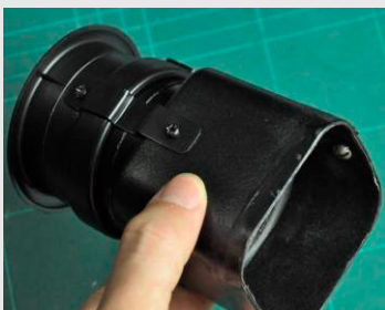
The inside are lined with black velvet paper to prevent glare and the outside spray painted matte black.
