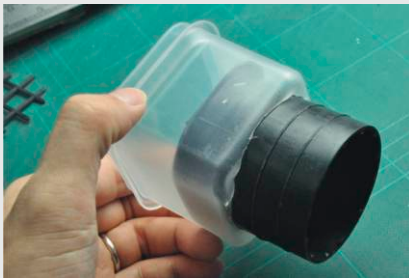
The rim of the clear plastic (A) will touch the LCD. Place the loupe temporarily at the end of (B).
