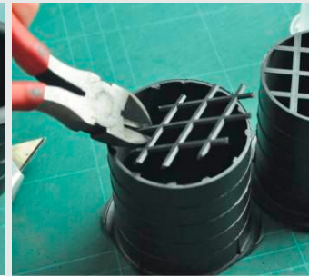
Remove the grill of black cylinder (B).
