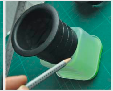
Trace the width of the black cylinder (B) onto the base of the plastic container (A).
