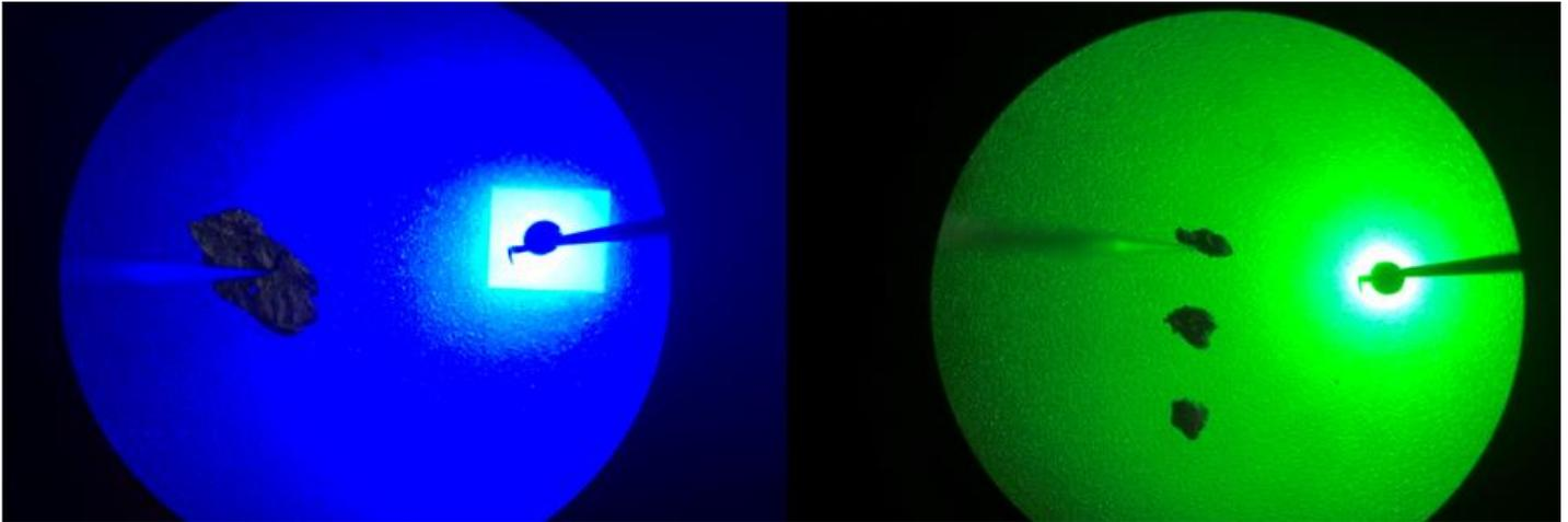
*Images: A preliminary demonstration of the electroluminescence from a two-colour (green on blue) cascade LED using BluGlass' RPCVD active-as-grown tunnel junction technology. These images are both from the same cascade LED wafer, with the electrical contacts configured to drive only the lower blue LED (left) and only the upper green LED (right).*
