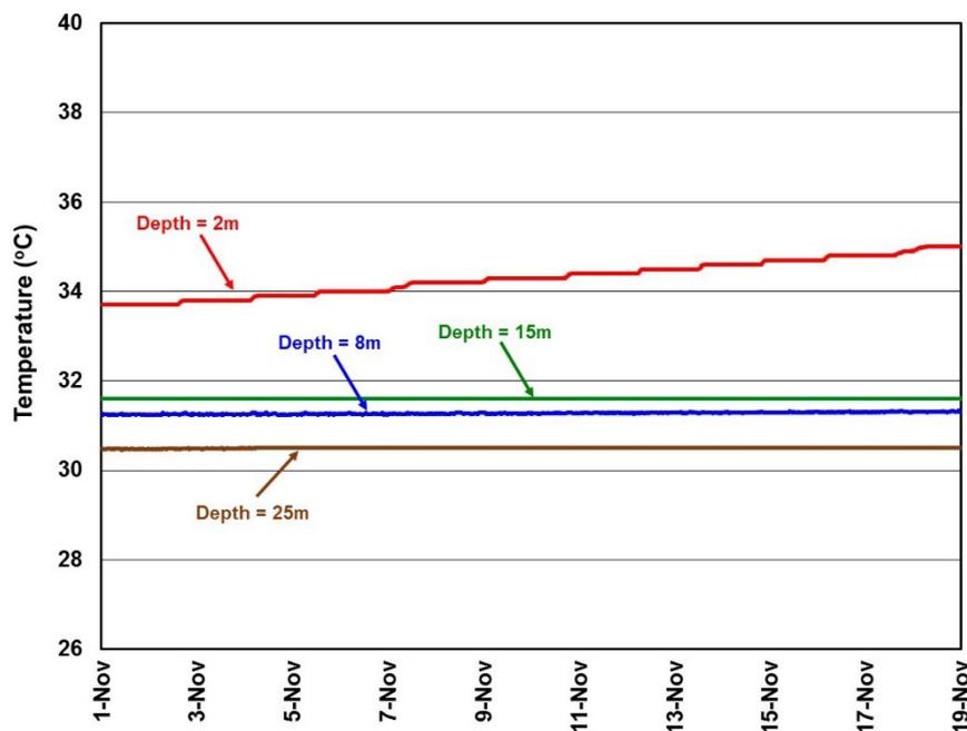
**Fig. 6. Temperature profile within the waste rock at selected borehole location**
