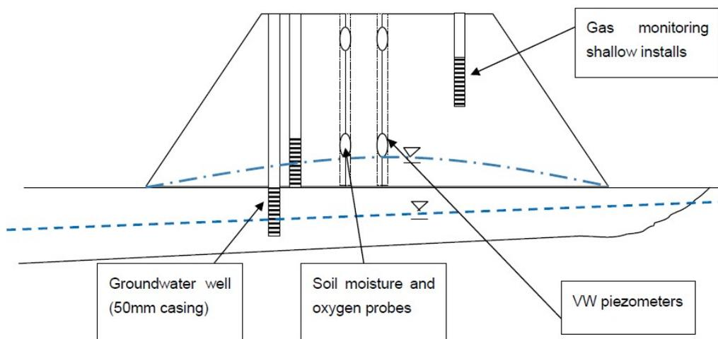
**Fig. 3. Conceptual layout of monitoring equipment**
