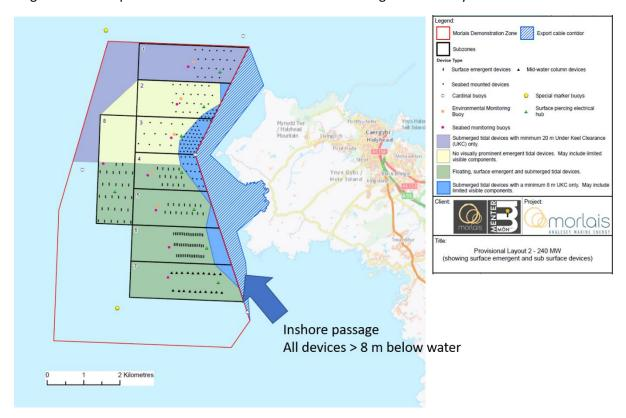
The area between the MDZ and the coast is termed the 'inshore passage' and is intended to give a 1 km zone with no emergent devices for passage of small boats (indicated dark blue in layout map).
