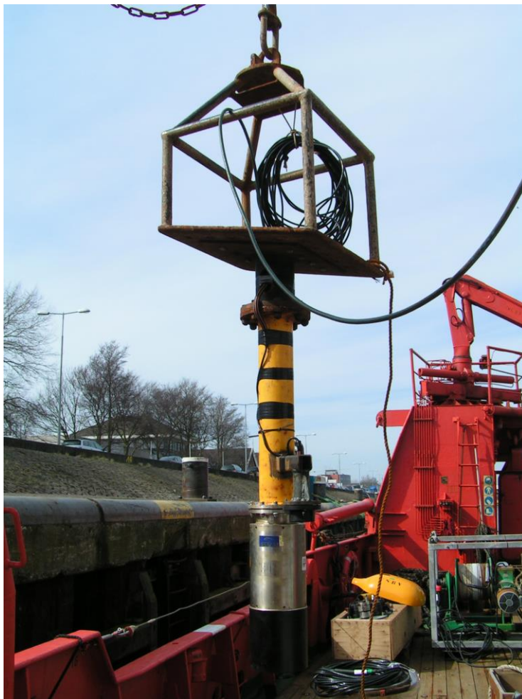
Moon pole carrier to install USBL, echosounder
