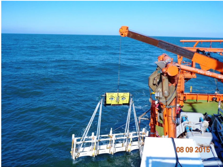
launch – recovery of GEOWING-SYSTEM, by use of ATLAS-CRANE SWL 2.5T
