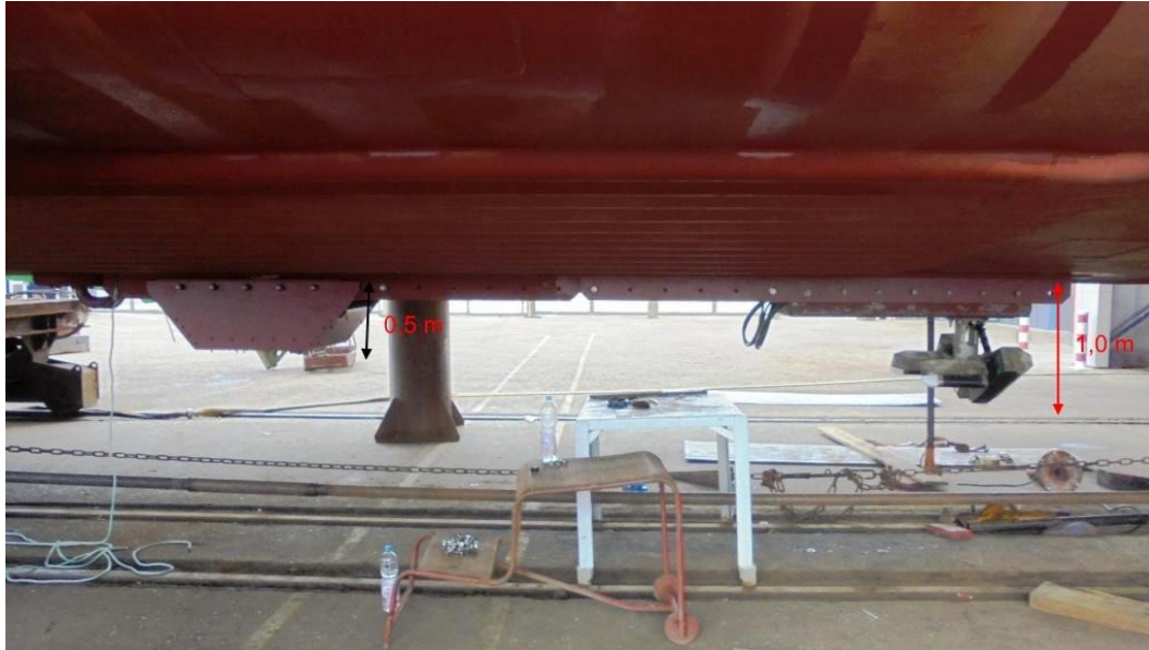
Under water rail system to install charterer equipment (MULTI BEAM EM 712)
