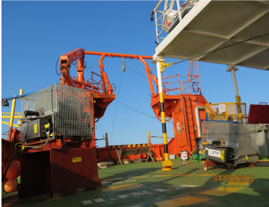
A-FRAME AFT SWL 3,0 T Height A-FRAME AFT below padeye 5000 mm Width A-FRAME AFT between legs 2300 mm Width A-FRAME AFT between foundation 4000 mm
