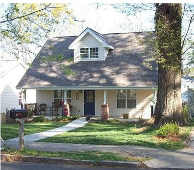
**Visitable Home**: This home was designed with visitability features in place and problems were avoided. With new construction, the walkway can be tied directly into the porch by grading the lot.
