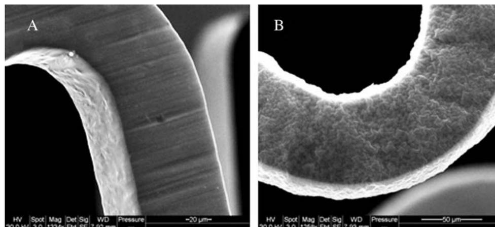
**Figure 1.** Scanning electron microscopy images of 316L stainless steel stent surface before and after electrodeposition of pBuOPy using CV.
