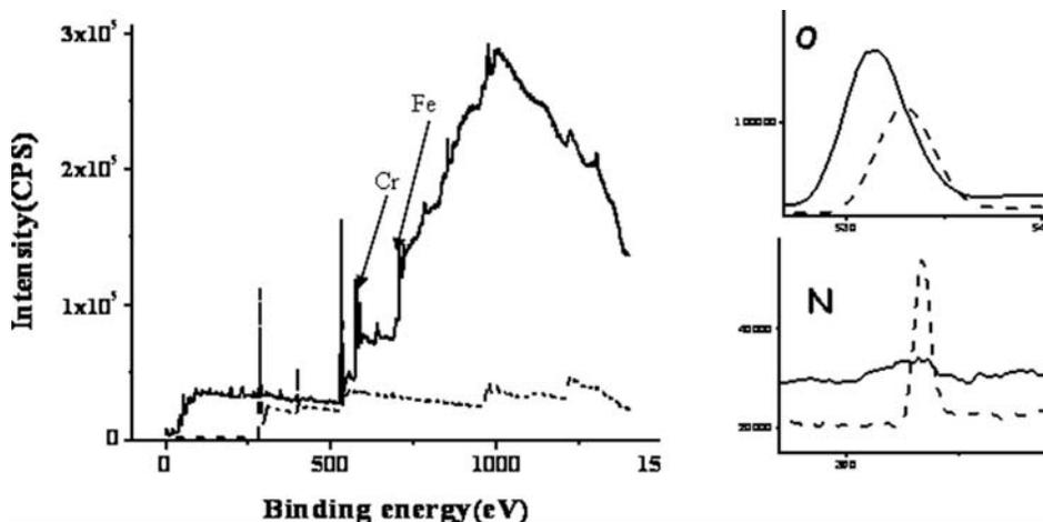
**Figure 3.** A wide survey scan, low resolution XPS (0–1400 eV) of bare (—) and pPPA coated (—) (~0.4  $\mu\text{m}$  thick) stainless steel plate. Close up (on the right) to oxygen (O) and nitrogen (N) signals detected on bare (—) and pPPA coated (—) stainless steel surfaces by high resolution XPS.
