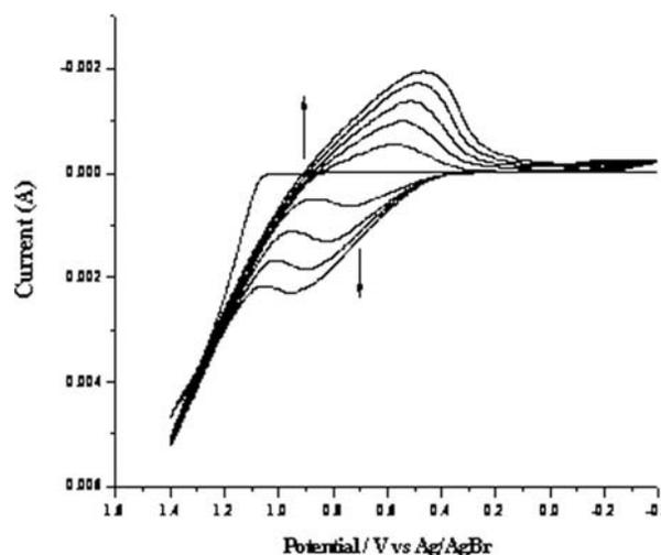
**Figure 2.** CV of 0.1M of pBuOPy in 0.1M acetonitrile solution of TBATFB at scan rate of 0.1 V/s (E vs. Ag/AgBr) on stainless steel plate.
