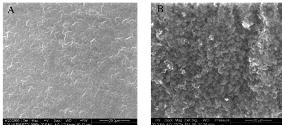
**Figure 8.** SEM images of the p(BuOPy:PPA) coating before drug loading (A) and after (B) drug release to phosphate buffer solution with 0.3% SDS up to 3 weeks. Scale bar represents 20  $\mu\text{m}$ .
