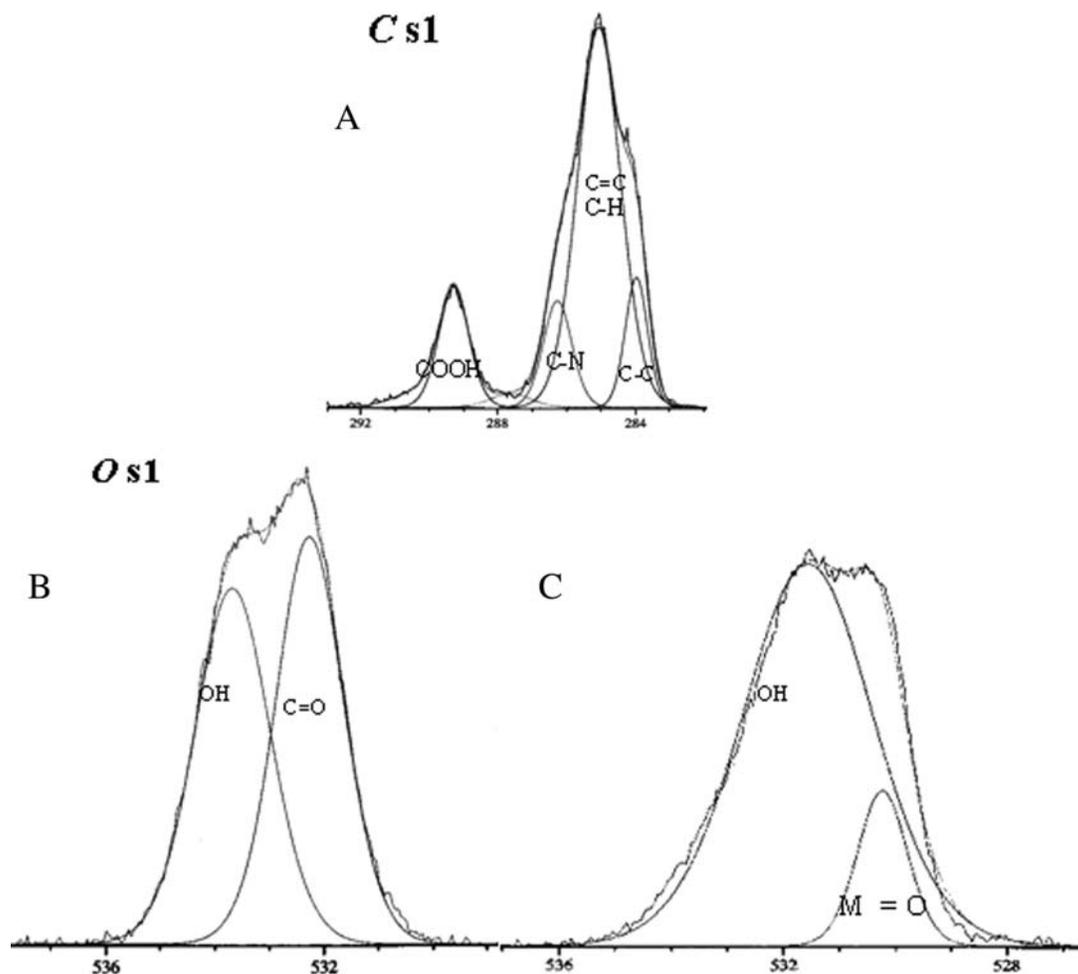
**Figure 4.** High resolution XPS spectra of C1s (A), O1s (B) core level region of pPPA coated stainless steel plate, and O1s (C) of bare stainless steel plate.
