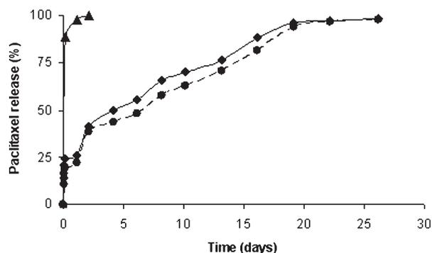
**Figure 7.** *In vitro* release profile of paclitaxel from bare metal stent ( $\blacktriangle$ ), PBUOPy ( $\blacklozenge$ ), and P(BUOPy:PPA) (9:1) ( $\blacksquare$ ), coated stents into 0.1M buffer phosphate pH = 7.4 with 0.3% SDS at 37 $^{\circ}\text{C}$ . Each symbol represents the cumulative amount of drug released, detected by HPLC.
