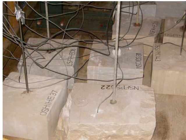
Figure 2: Stone-anchor assemblies with embedded sensors in the environmental chamber.
