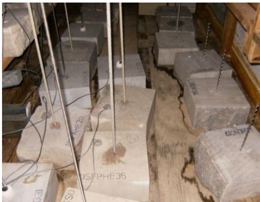
Figure 6. Stone-anchor assemblies with embedded sensors in the environmental chamber.
