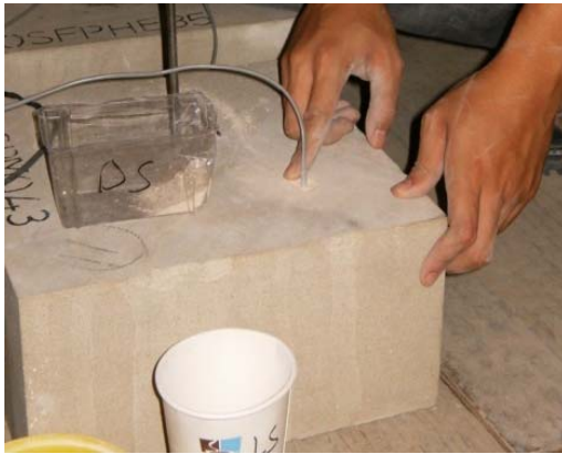
Figure 5. Duff gauge sensor installation; original stone dust used to fill the hole.
