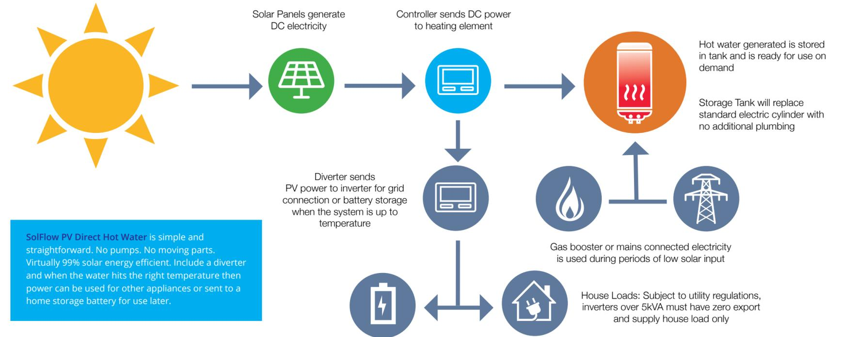
SolFlow PV Direct Hot Water is simple and straightforward. No pumps. No moving parts. Virtually 99% solar energy efficient. Include a diverter and when the water hits the right temperature then power can be used for other appliances or sent to a home storage battery for use later.
