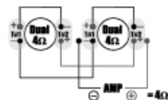
Series/Parallel Wiring for Two Dual Voice Coil 4Ω Subs
