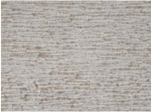
FINE ADZE min thickness - 1.5" / 38 mm
