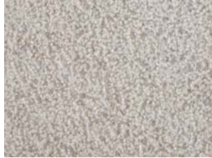
BUSH HAMMER min thickness - 1.5" / 38 mm
