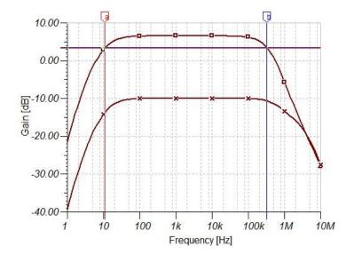
**Bandwidth:** 3dB bandwidth of both inputs 'A' and 'B' is 10Hz to 300KHz Studio Quality and beyond. **Mixer:** Simple High level transistor mixer. Low latency, non op-amp design. Max input at min gain = 3V p-p
