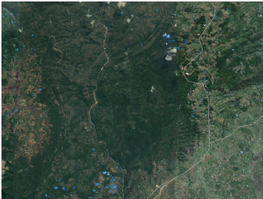
Figure 9: Outputs from the prototype deforest tool, showing 'confirmed' deforestation events in blue for the year 2017 in the vicinity of Moribane forest reserve in Central Mozambique, one of the locations selected to perform fieldwork.
