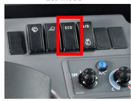
Switching to Eco mode controls the engine speed efficiently whilst letting you use less fuel as you work, reducing it by 300 rpm
