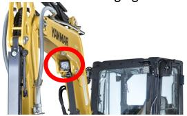
In order to work safely, efficiently and with accuracy in the darkness, the ViO57-6 is equipped with a powerful LED work lamp. The lamp, positioned in the inner part of the boom gives a wide coverage of light, whilst still reducing energy consumption and preserving battery life.
