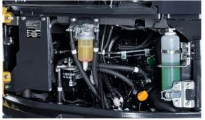
Upgrading of the powerline components (engine, hydraulic pump and control valve) will give users higher performance levels. Making heavy duty jobs in confined areas a much simpler task. Also making the digger more efficient on all jobs.
