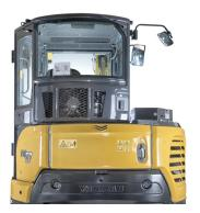
The cab is mounted on an innovative and sophisticated vibration reducing system. These mounts not only reduce the vibration levels felt by the operator but also the noise levels have been significantly reduced as well.
