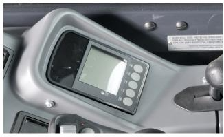
This new interface allows you to manage working time, daily maintenance checks and to programme interventions.
