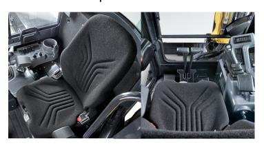
The wide, comfortable seat is fitted with air suspension as standard. It allows the operator to find their optimal working position by moving up or down and back or forth using the attached levers. The air suspension also reduces shocks and vibrations.
