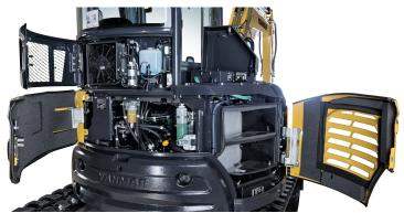
Large, lockable access hood give easy access to maintenance points. All major elements including; air filter, radiator, refuelling pump, battery, fuel tank, alternator, water separator and engine oil dipstick are located under the rear and side panels.
