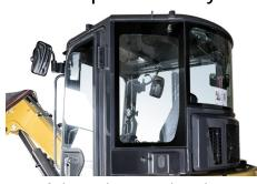
The shape of the cab provides the user with an optimal 360° of the surrounding area. This had reduced the rear blind spot to a minimum. The machine is also equipped with three adjustable mirrors, allowing the operator to control the work area without having to move from their seat.
