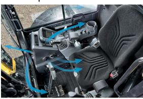
The cab now houses six air vents, optimally located to improve air circulation. A fresh air function has been added and both air filters are more easily accessible, improving greatly comfort on hot days.
