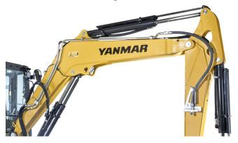
A new boom design has improved the lifting force by 10%. This new design also reduces the weight of the boom by 40%, increasing the stability.
