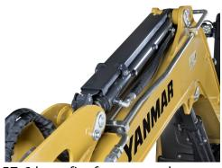
The ViO57-6 benefits from complete protection of all its boom, arm and bucket cylinders. All of the cylinder tubes and rods are protected by a spring type steel plate. This offers the highest protection and reduces the chance of damages and resultant downtime.
