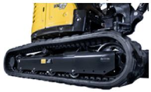
The redesign of the undercarriage has also contributed towards a reduction of the machines height to 2.54m. This again helps the machine be more compact but will also aid in transportation.
