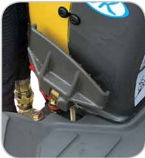
Retractable pedals (PTO pedal and swing control pedal)
