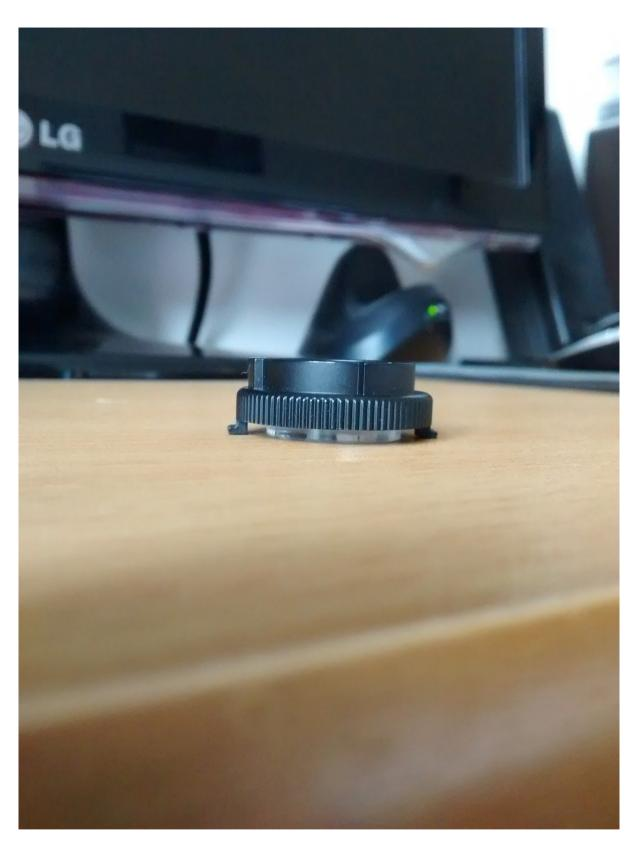
Refit the bezel and lens to the LAM aperture by aligning the tangs to 12 and 6 o'clock positions and turn anticlockwise to lock in.
