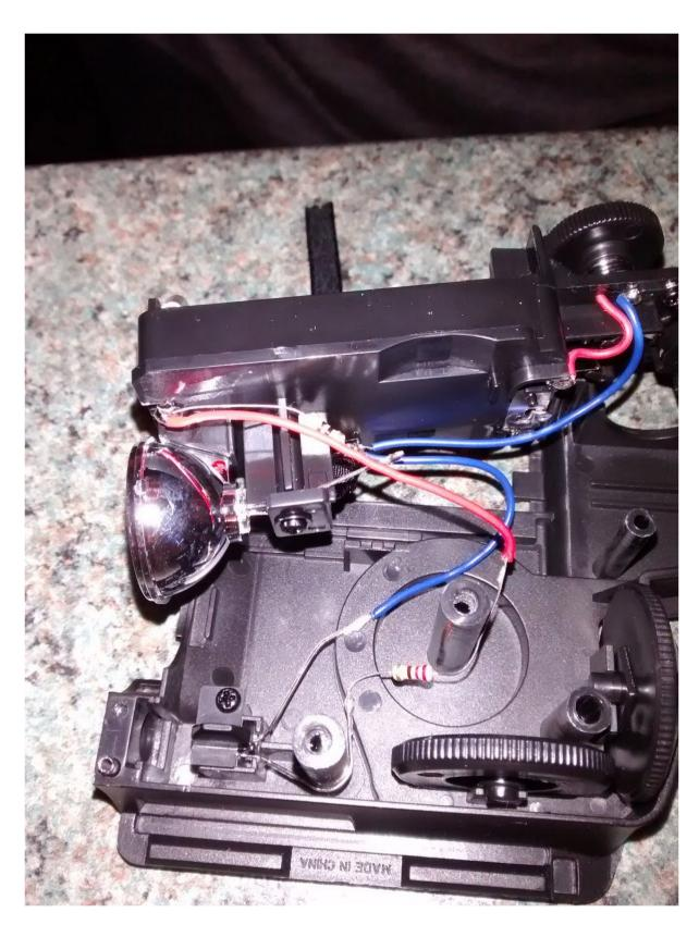
Unscrew the small plate holding the legs of the LED to enable it's removal.
