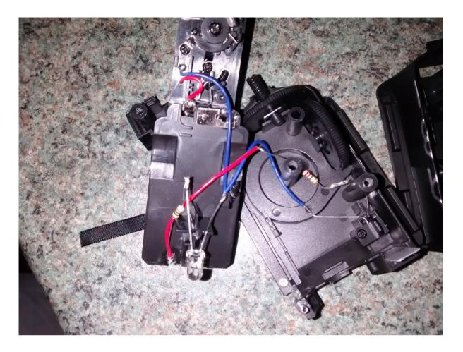
Ok, now using the side cutters snip off the first resistor leg (lamp LED) just where the red wire enters from the battery compartment.
