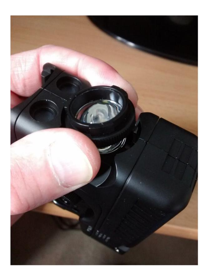
Open and remove the battery compartment lid. Remove the three Allen screws securing the body together.
