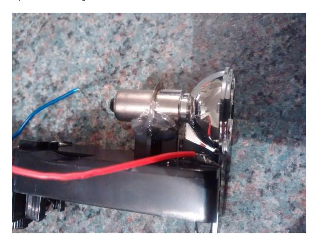
Now we're ready to get soldering, so warm up your iron. Solder one wire to the main body of the LED module and the other to the tail cap.
