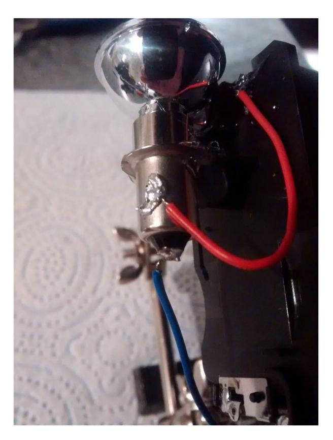
I haven't been specific here about which way round to connect red and blue because the LED I linked to at the start is non polarity, so it shouldn't matter. You can now fit the batteries temporarily and test the light.
