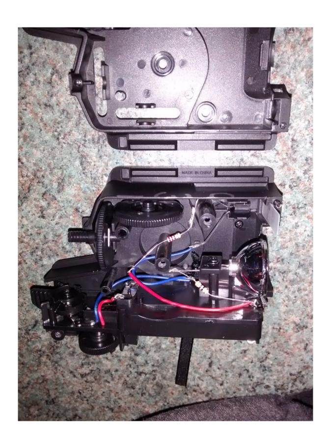
Now, we will be removing the LED from the lamp, both resistors and one blue wire. The LED 'fake laser' in the top will be disconnected out of circuit but can be left in place.
