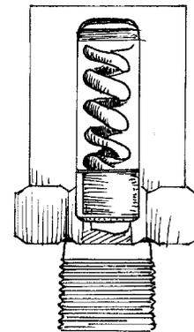
**Figure 9. Pressure-relief Valve**
