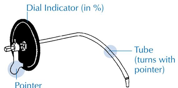
**Figure 10. Rotary Gauge**
