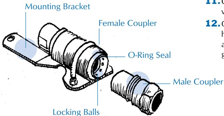
**Figure 13. Breakaway Coupler**
