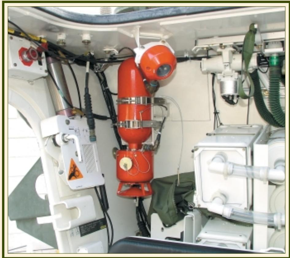
digital signals from the system detectors, manual activation devices and external status switches; process the inputs; activate the fire extinguishers according to the system logic including selection of properly charged and connected cylinders and enabling backup extinguisher activation; control indication and annunciation devices (audiovisual); and enable performance of system maintenance and trouble shooting according to diagnostic information continuously gathered from the system components.
