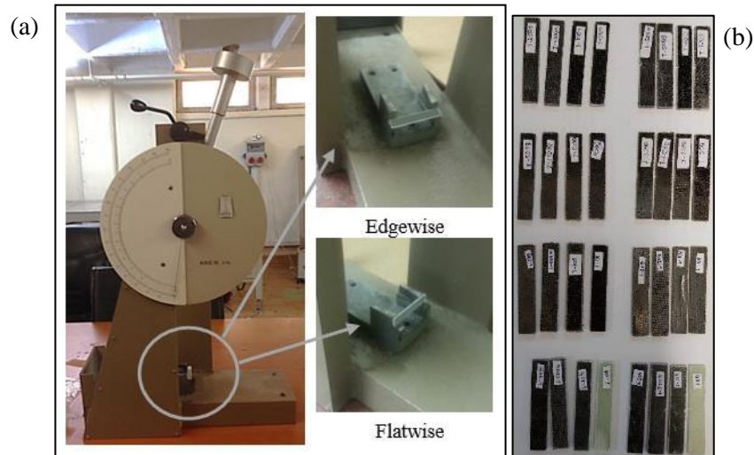
Figure 2. (a) Charpy impact test device and sample positions, (b) Test samples.
