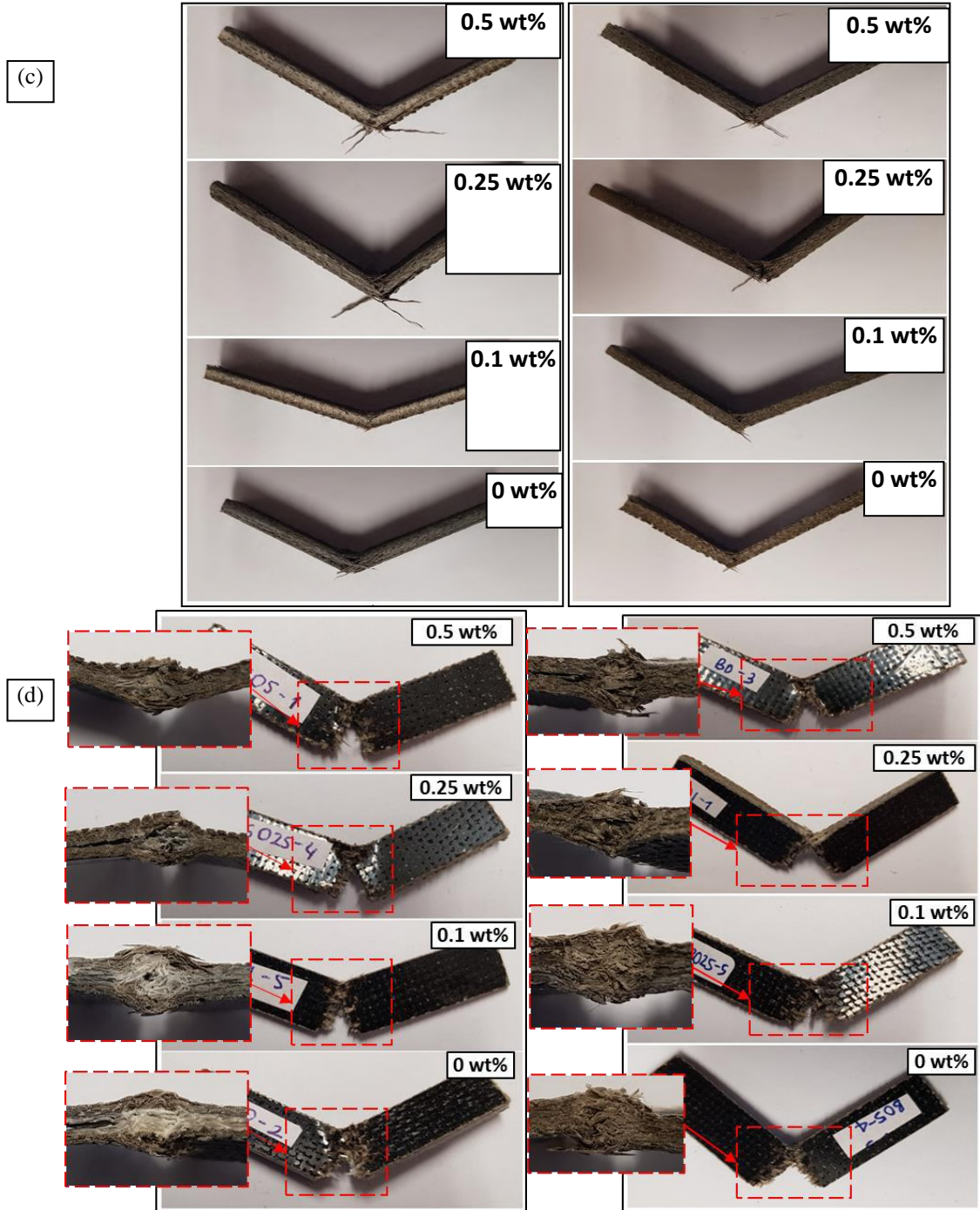
Figure 4. Photos of (a) GFR, (b) GBFR, (c) BGFR and (d)BFR notched/unnotched composite samples after Charpy impact tests.
