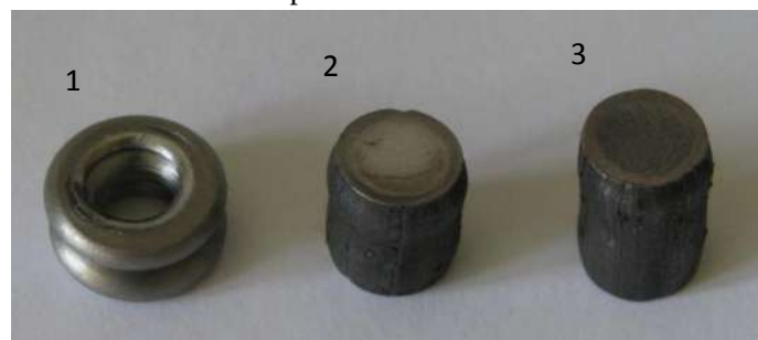
Figure 13. Shape variations of compression samples with core material.
