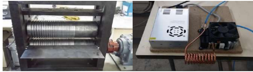
Figure 2. Roll forming machine and induction heating system.
