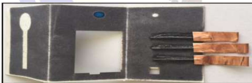
Figure: Pencil Lead electrode in paper microfluidic chip fabrication
