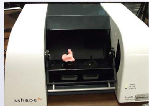
Figure 1: ScanIt Legato 2 with earmold impression loaded in scanner
