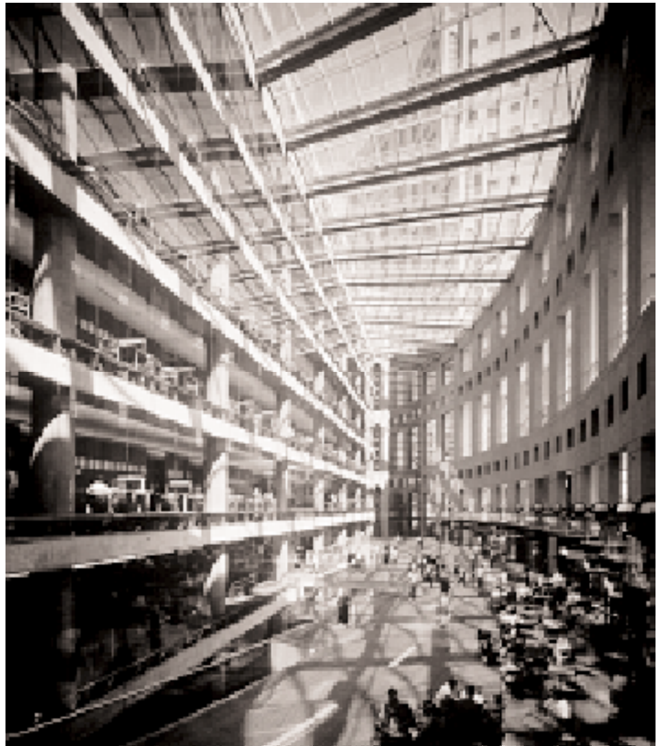
Figure 1. New Spectrally Selective Glazings at the Vancouver Library Atrium (The atrium offers viewers a clear connection to the outdoors without the uncomfortable heat gains associated with clear glass. The glazing is double-pane selective coating on clear glass: T_v=0.70 , SHGC=0.37 .)
