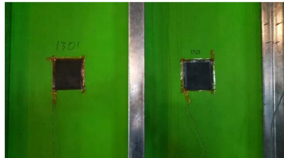
Figure 3. Interior Heat Flux Sensor Installation
