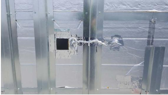
Figure 4. External Heat Flux, Temperature and Pressure Installation
