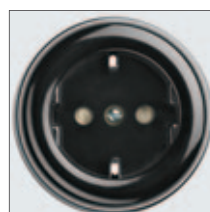
SURFACE-MOUNTED OUTLET DUROPLAST 16 A, AC 250 V, IP 20 62 mm Ø, height above surface 49 mm. Duroplast housing with integrated child protection. With spring clip. Order-no. 184199
