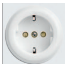
SURFACE-MOUNTED OUTLET DUROPLAST 16 A, AC 250 V, IP 20 62 mm Ø, height above surface 49 mm. Duroplast housing with integrated child protection. With spring clip. Order-no. 184199
