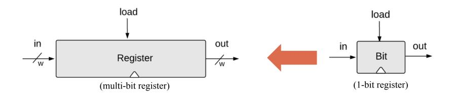
A w-bit register can be created from an array of w 1-bit registers.
