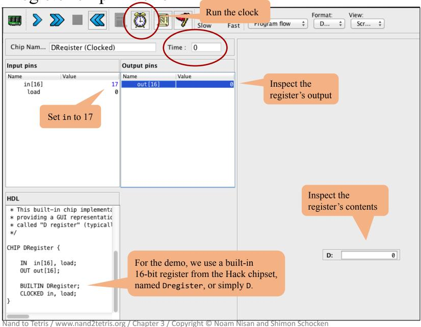
Register chip in action Run the clock Slow Fast : rrogram flow Chip Nam... DRegister (Clocked) Time: 12 **Output pins** Input pins Value Value Name Name Inspect the in[16] 17 out[16] load register's output
