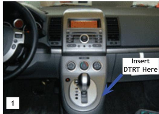
**STEP 2.** Once the shifter bezel is out of the way, insert the DTRT between the dash molding and the climate control bezel. Use the DTRT again in a twisting motion to release a series of four (4) retainer clips securing the climate control bezel to the dash. Do NOT disconnect the climate control wiring; simply allow the bezel to hang off to the side out of the way.
