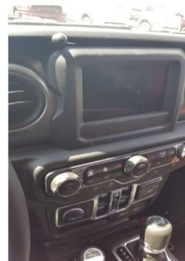
Step 1: Use the DTRT to remove the bezel with radio and climate controls. There are clips that hold this on. (Photo #1)
