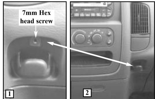
**STEP 2.** Remove four (4) 7mm hex head screws from the four (4) corners of the radio. Slide the radio out of its cavity and let it hang down. It is **not necessary** to disconnect the wiring to the radio.
