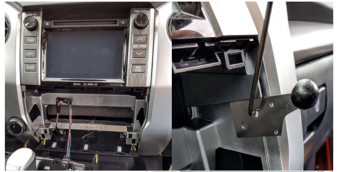
Step 2: Place the mount just below the plastic piece that indents in the opening. The mount should be tight to the bottom of this. The mount's 2 smaller holes should line up with the edge of the trim (Pic2). Mark the 2 larger screw holes and drill pilot holes or using cordless drill attach mount using screws provided.
