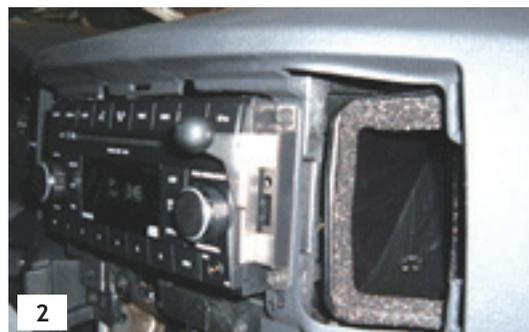
**STEP 3.** Remove the two Phillips screws to the right of the radio and carefully set them aside. Place the VSM G3 flush and to the right of the radio exactly in place as pictured in Photo #2. Replace the two Phillips screws over the pilot holes in the legs of the VSM G3 and tighten the VSM G3 evenly and securely in place as pictured.
