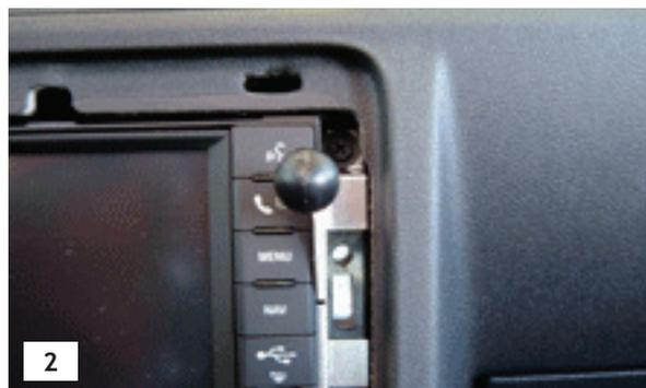
**Step 3:** Once the VSM G3 is flush and secured to the right side of the radio, replace the radio bezel back into its secured original position. You have successfully installed your VSM G3!
