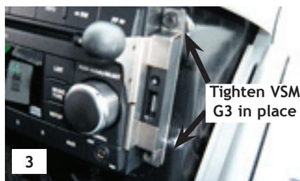
**STEP 4.** After the VSM G3 is flush and tightened, begin to assemble the dash back in the reverse order in which it was disassembled. You have successfully installed your VSM G3.
