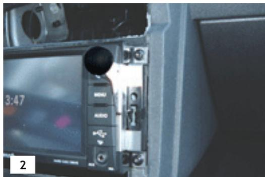
**STEP 3.** Once the VSM G3 is flush and secure, place the dash back together again in the reverse order in which it was dismantled. You have successfully installed your VSM G3.
