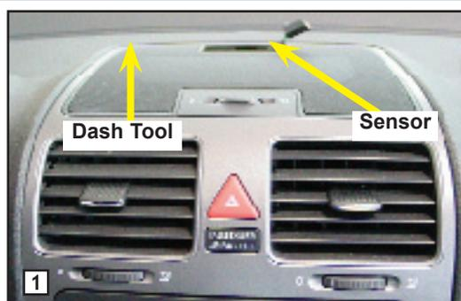
STEP 2. Slide dash tool behind air vent trim bezel in the back, left corner as before. **Photo 1.** Release clip and work the tool clockwise around bezel, pulling outward until bezel is free. Set bezel aside.
