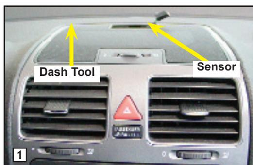
STEP 2. Slide dash tool behind air vent trim bezel in the back, left corner as before. **Photo 1.** Release clip and work the tool clockwise around bezel, pulling outward until bezel is free. Set bezel aside.
