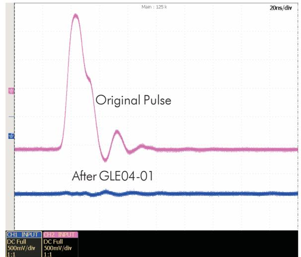
Impulse response of GLE04-01 (into 10 Ohms load)
