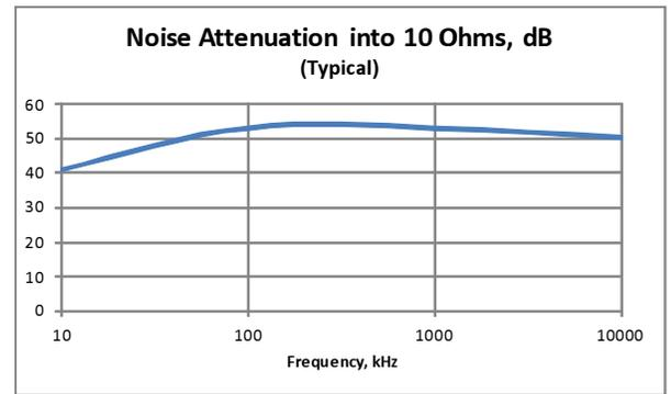
Frequency response of GLE04-01 (into 10 Ohms load)
