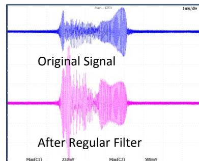
Figure 6. Regular EMC filter amplifies noise
