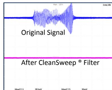
Figure 7. CleanSweep® EMI filter reduces noise
