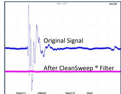
Figure 9. Attenuation of a typical transient signal by CleanSweep® EMI Filter
