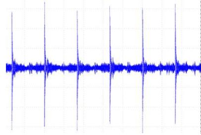
Figure 2a. Typical periodic spikes on power lines
