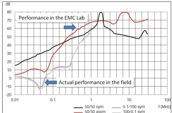
Figure 5. Typical attenuation of a regular EMC filter
