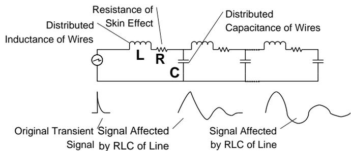
Figure 3. Transformation of a short pulse by power network
