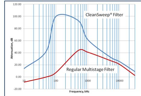
Figure 8. Attenuation of CleanSweep® EMI filter in 1/100 Ohms environment
