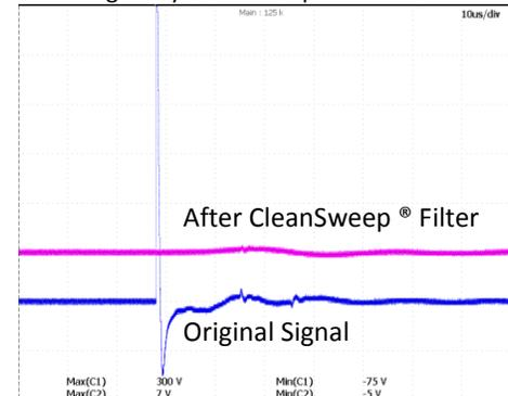
Figure 10. Attenuation of a power line surge signal by CleanSweep® EMI Filter
