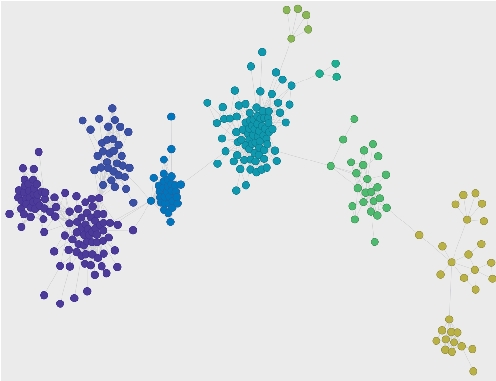
Figure 1.3: Network communities and modularity. Personal Facebook network of the author of this PhD Thesis. Five important communities are detected and highlighted in different colors. Nevertheless, different partition algorithms can lead to the detection of different communities. The network modularity Q allows to objectively assess which of the algorithms leads to the best partition, at least when compared with the randomized version of the network (still maintaining the number of communities).
