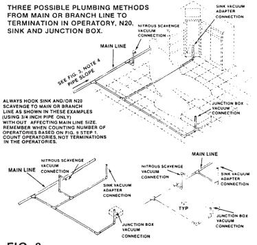
FIG. 8 N2O AND SINK VACUUM CONNECTIONS
