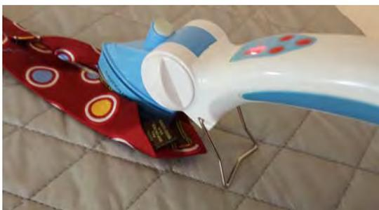
3) **Place the tag on the garment and press with the Petite Press for 6-8 seconds.** If you have enough heat and pressure you will see a little of the glue seep out around the edge of the tag - but just a tiny amount. The Petite Press will cover the tag completely. If you leave the iron on too long it will melt the adhesive too much and the tag won't stick.
